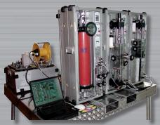
The obligation to obtain data on field as fast as possible for its exploitation led us to realizein collaboration with and at the request of petroleum companies a transportable unit for on site PVT analysis.
